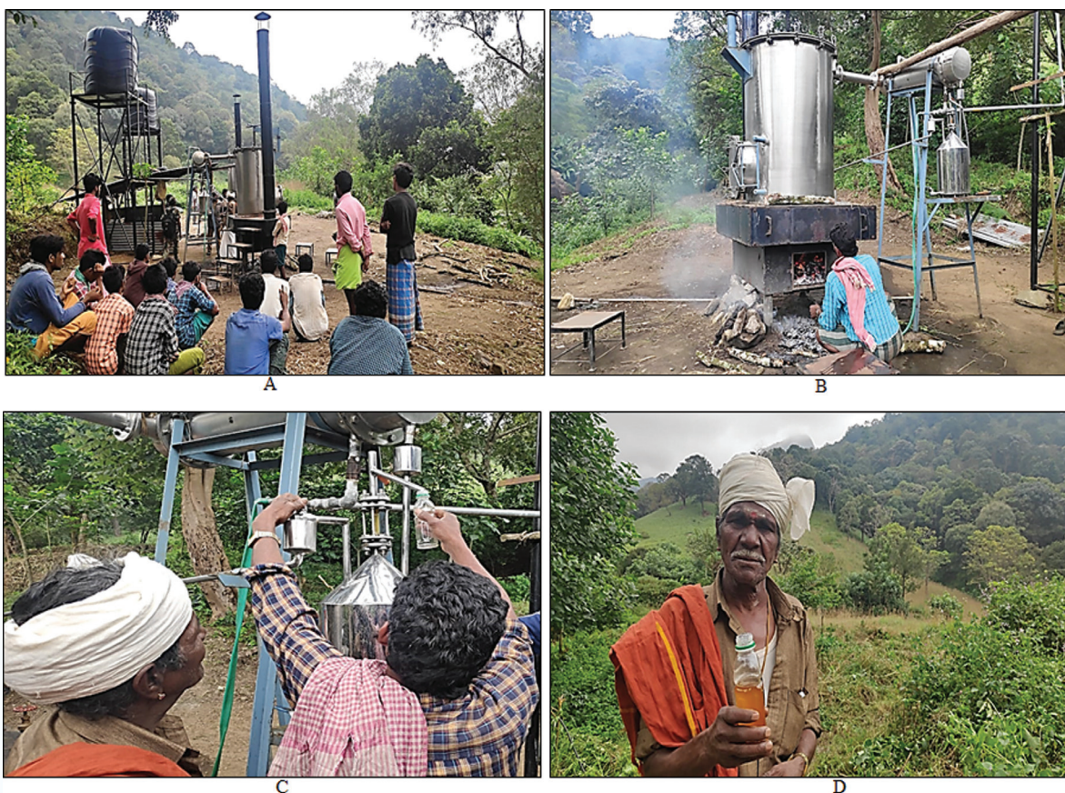
Image: Distillation unit installed under CSIR-Aroma Mission at Anamalai Tiger Reserve Extraction of lemongrass oil by tribes ; A) Distillation unit view, B) Distillation unit operated by a trained farmer, C) Oil collection process and D) farmer holding collected Lemongrass oil.
