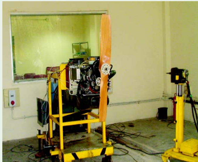
Wankel engine fitted with a propeller on the NAL Test Bed
