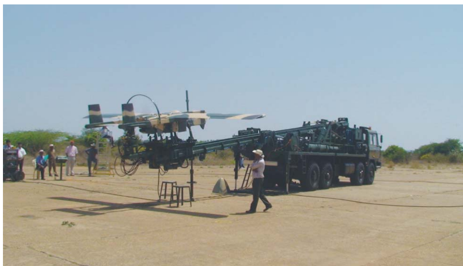
NISHANT , fitted with the indigenous Wankel engine, on the Hydro-Pneumatic Launcher
