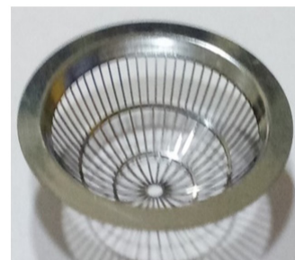
Ultrafast Laser micromachining facility at ARCI (50- 100 fs, 800, 400 & 266 nm, and 100 ns, 527 nm, at 10 kHz) and the 3-D control grid created using such system
